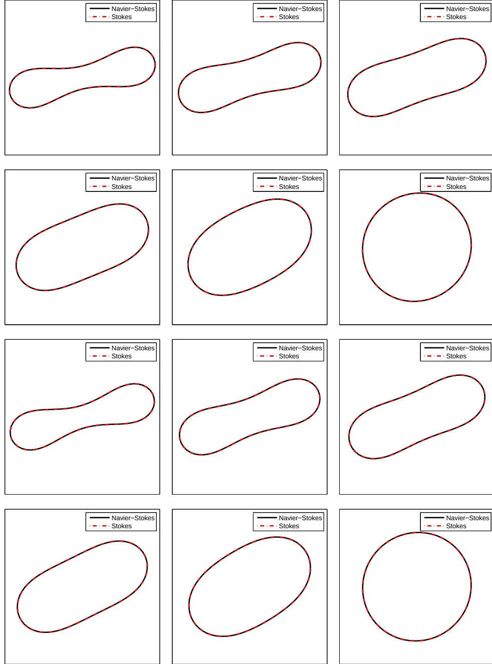
Figure 3.3: The equilibrium inclination angle of a single cell with swelling ratio s^*=0.481 , 0.6, 0.7, 0.8, 0.9, 1.0. Degree of confinement is R_0/w=0.8 for top two rows and 0.4 for the bottom two rows.
